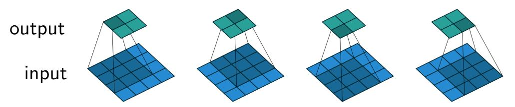
Figure 2.1: (No padding, unit strides) Convolving a  $3 \times 3$  kernel over a  $4 \times 4$  input using unit strides (i.e., i = 4, k = 3, s = 1 and p = 0).
