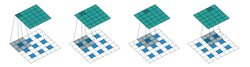
Figure 4.6: The transpose of convolving a  $3 \times 3$  kernel over a  $5 \times 5$  input padded with a  $1 \times 1$  border of zeros using  $2 \times 2$  strides (i.e., i = 5, k = 3, s = 2 and p = 1). It is equivalent to convolving a  $3 \times 3$  kernel over a  $3 \times 3$  input (with 1 zero inserted between inputs) padded with a  $1 \times 1$  border of zeros using unit strides (i.e., i' = 3,  $\tilde{i}' = 5$ , k' = k, s' = 1 and p' = 1).
