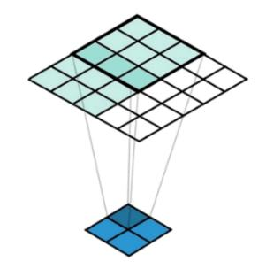
Figure 4.5: The transpose of convolving a  $3 \times 3$  kernel over a  $5 \times 5$  input using  $2 \times 2$  strides (i.e., i = 5, k = 3, s = 2 and p = 0). It is equivalent to convolving a  $3 \times 3$  kernel over a  $2 \times 2$  input (with 1 zero inserted between inputs) padded with a  $2 \times 2$  border of zeros using unit strides (i.e., i' = 2,  $\tilde{i}' = 3$ , k' = k, s' = 1 and p' = 2).
